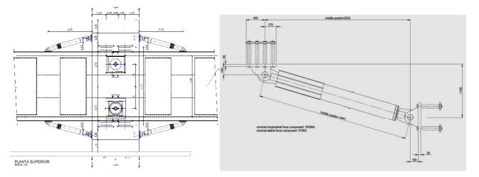
Figure 2 On the left side- Top view on fixed delta pier axis with spherical bearing in centre, re-centring spring rubber bearings and viscous dampers [1]- On the right side- Viscous dampers with support brackets[3]
