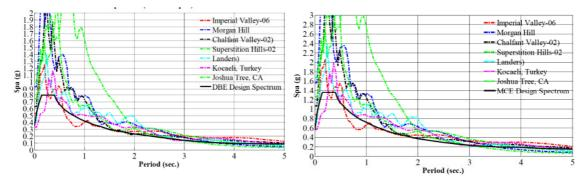
Figure 6 Horizontal pseudo acceleration spectrum (5 % damping) for DBE(on the left) and MCE (on the right)-level ground motion
