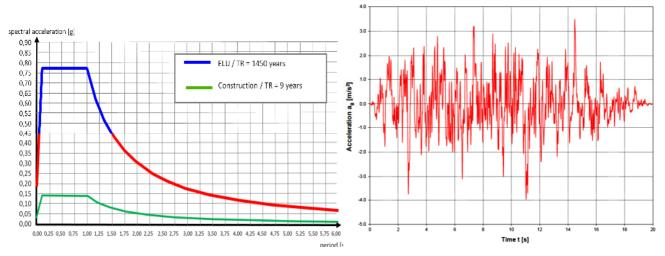
Figure 1 Response spectrum for 1475 years return period; on the right artificial accelerogram [2]
