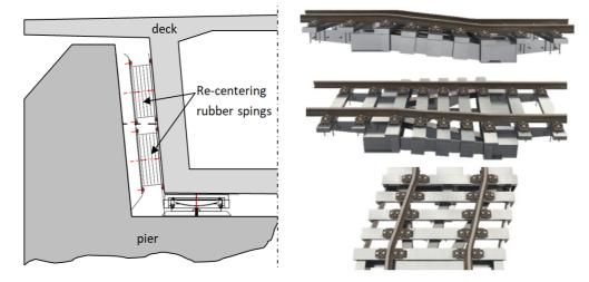
Figure 3 On the left side: Arrangement of re-centering rubber springs on fixed axis between deck an pier top concrete buffers; sample on top of delta pier [4], on the right side: Cross Tie enables longitudinal displacements with lateral, torsional and vertical off-set
