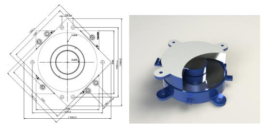
Figure 7 Design of the biggest SIP D isolator
