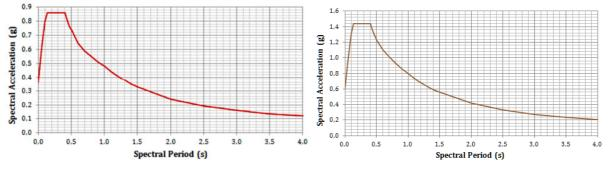
Figure 5 Horizontal specific spectra for 475(on the left) and 2475 (on the right) years return period (5 % damping)
